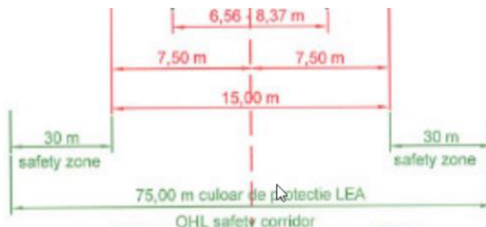
Figure 3-11: The 400 kV OHTL Safety Zone
