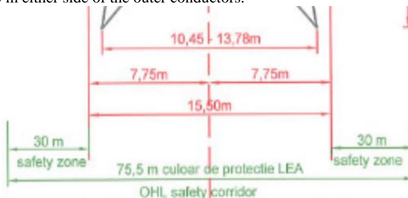
Figure 3-13: The 400 kV OHTL Safety Zone
