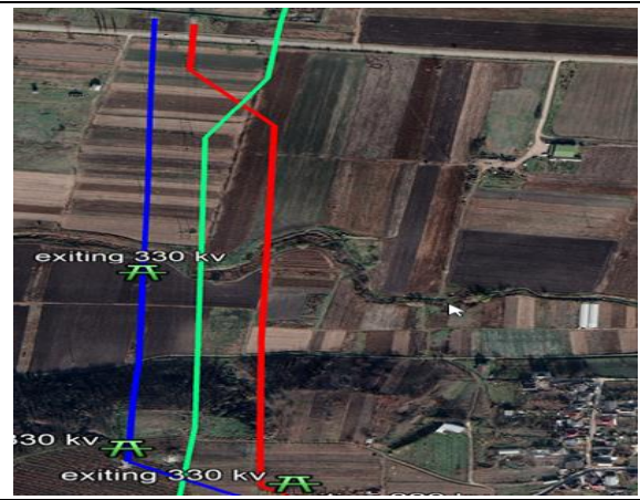
Fig. 5-3: The 400 kV OHTL passes on the territory of the com. Bacioi (green line)
