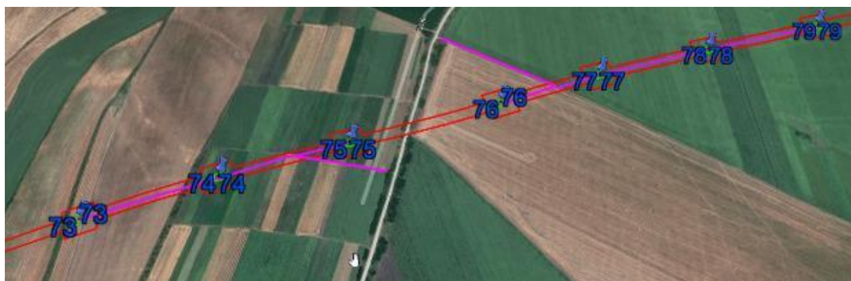
Figure 3-16: Access road to the tower's foundations (pink colour)
