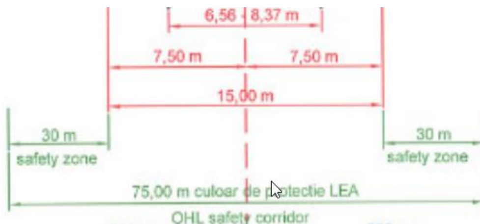
Figure 3-17: The 400 kV OHTL Safety Zone
