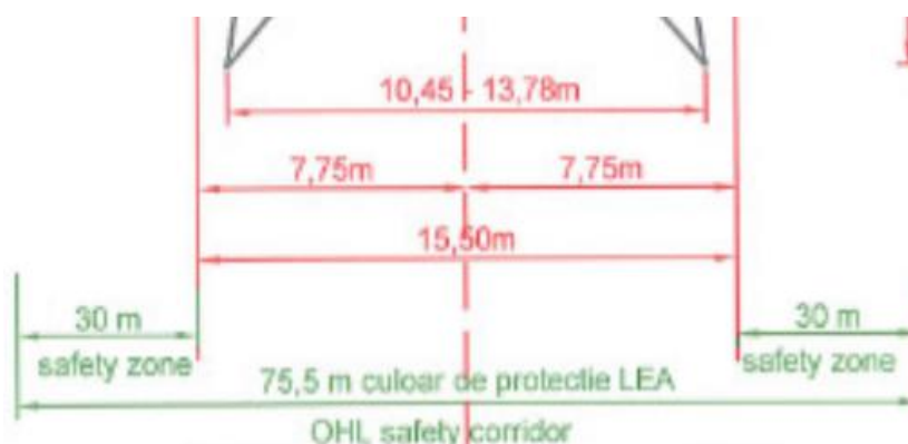
Figure 3-11: The 400 kV OHTL Safety Zone
