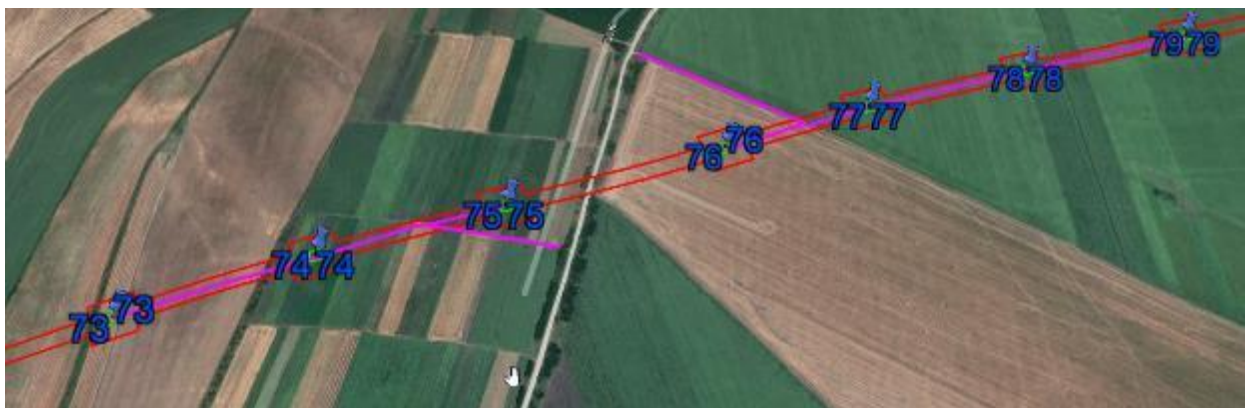
Figure 3-10: Access road to the tower’s foundations (pink colour)
