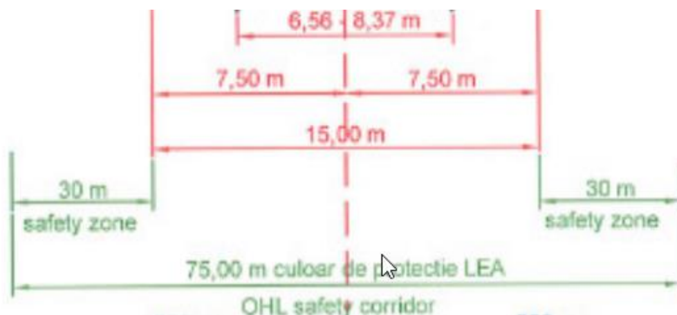
Figure 3-17: The 400 kV OHTL Safety Zone
