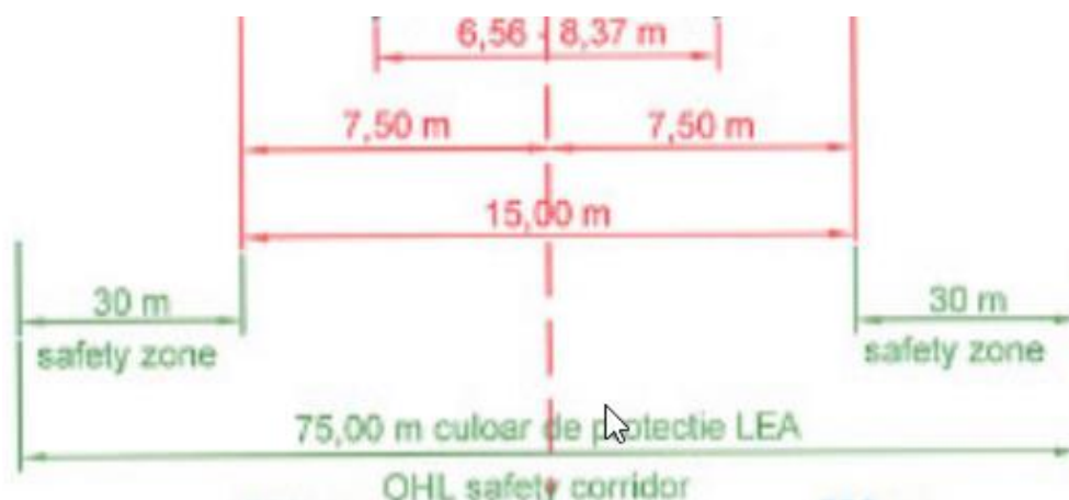
Figure 3-11: The 400 kV OHTL Safety Zone
